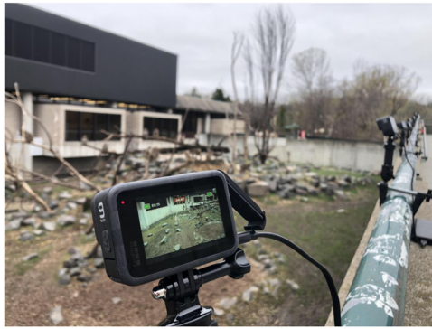
FIGURE 1 Camera tracking system at the Minnesota Zoo. Relatively affordable cameras, such as GoPro cameras, when combined with computer vision tracking software, can provide estimates of pose, although they depend on having long-term access and a safe vantage point
